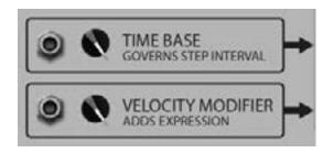
Time Base. If the Beat is set to a note length, the Time Base CV Input nudges the sequencer forward or back by up to 1 step. If the Beat is set to CV, the Time Base CV directly controls the play head position of the main sequencer. If the Beat is set to CVJ, the Time Base CV controls the rate of playback, where -1 will play back in reverse 16 steps per
