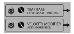
Time Base. If the Beat is set to a note length, the Time Base CV Input nudges the sequencer forward or back by up to 1 step. If the Beat is set to CV, the Time Base CV directly controls the play head position of the main sequencer.
